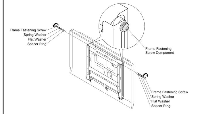
\* Confirm that all of the parts are securely fastened and do not rattle and loose.
